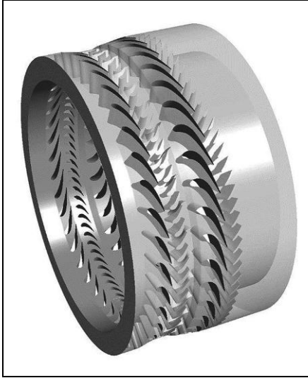
Figure 6. Overall geometry of GE-E 3 two-stage high-pressure gas turbine.
